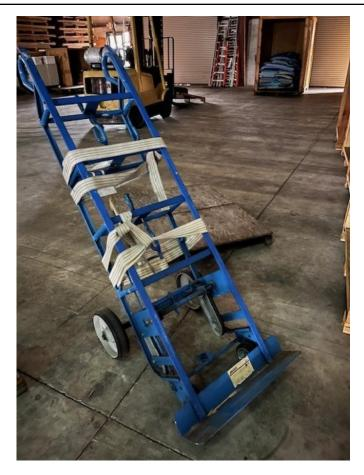
(Year: N/A) Description: Dutro Appliance Truck 66" high; retractable wheels; 1600 lbs. capacity
