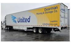
(Year: 2001) Description: 53 Ft Electronics/Spec Com Flat floor trailer with power tailgate
