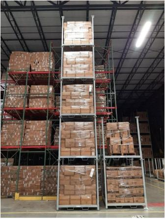
(Year: N/A) Description: Used Stack Racks, 60"x60"x70" tall, Stack up to 5 high 4000 lb. capacity
